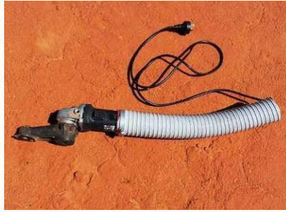
Figure 6. Arbortech® mini grinder with improvised dust cover (light grey) fitted to cover the handle and air intake. The dust cover is 45 cm long and held in place with a large hose clip.
