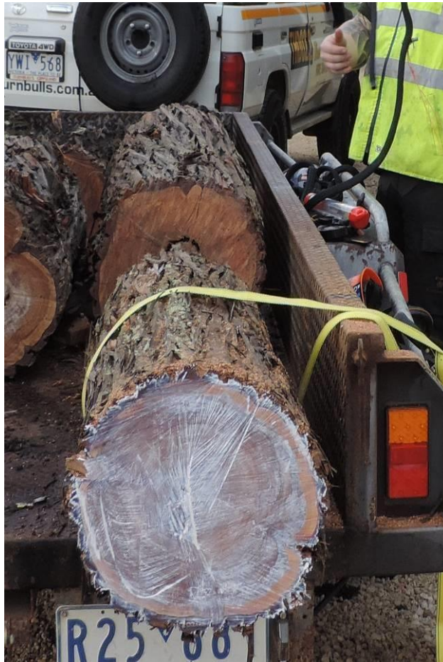
Figure 33. Log sealer painted on end-grain immediately after cutting to reduce splitting of Callitris log.
