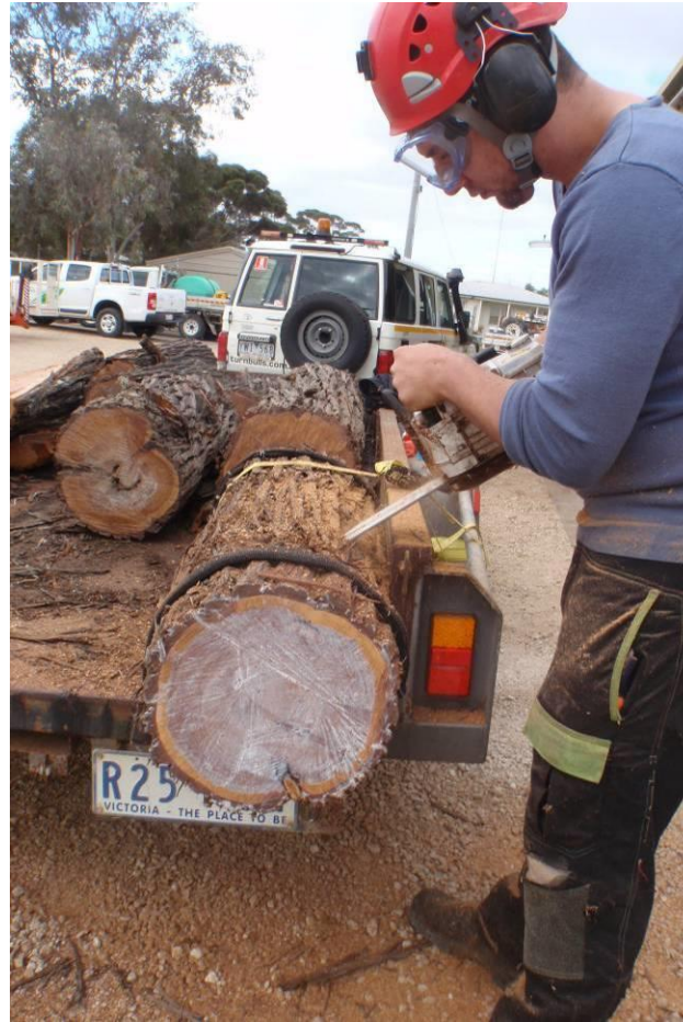
Figure 36. Longitudinal cuts angled at 45° to create a wedged section that will form the face plate.
