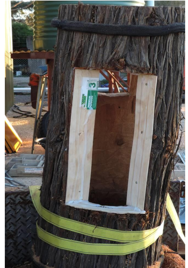
Figure 52. Plywood caulking planks tacked and glued into place. Wood glue placed on interior gluing surface ready for attachment of face plate.
