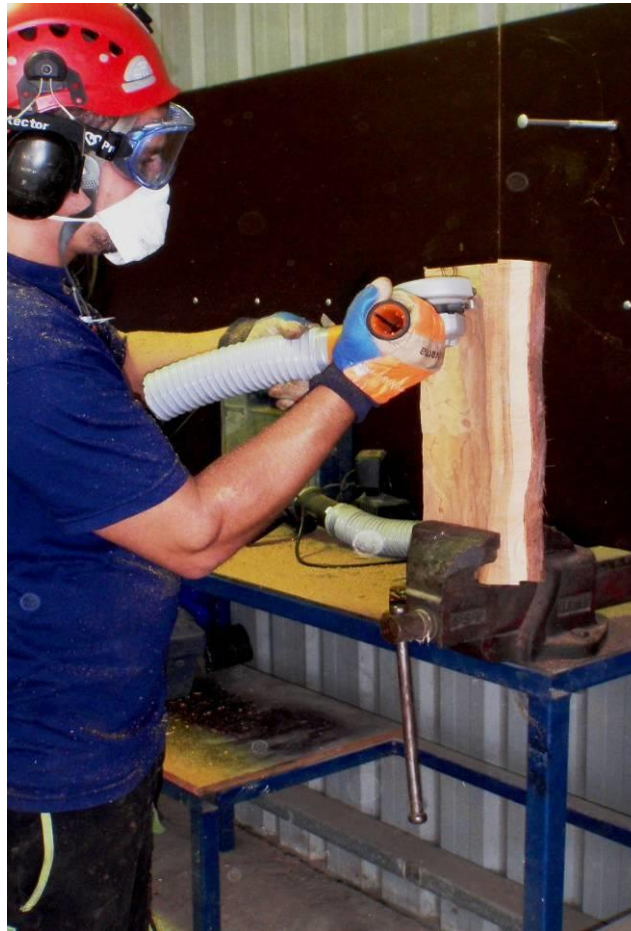
Figure 45. Where possible the face-plate is to be secured in a vice for ease of access and safety.
