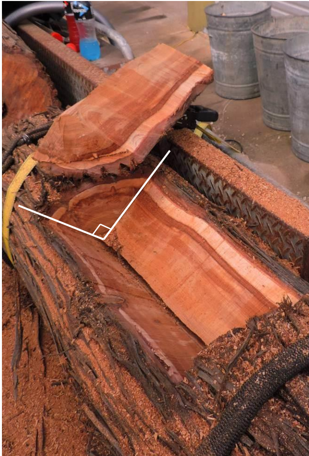
Figure 38. The wedge removed will later be carved to form a face-plate. Note the 90° angle of the narrow section removed for the face plate.
