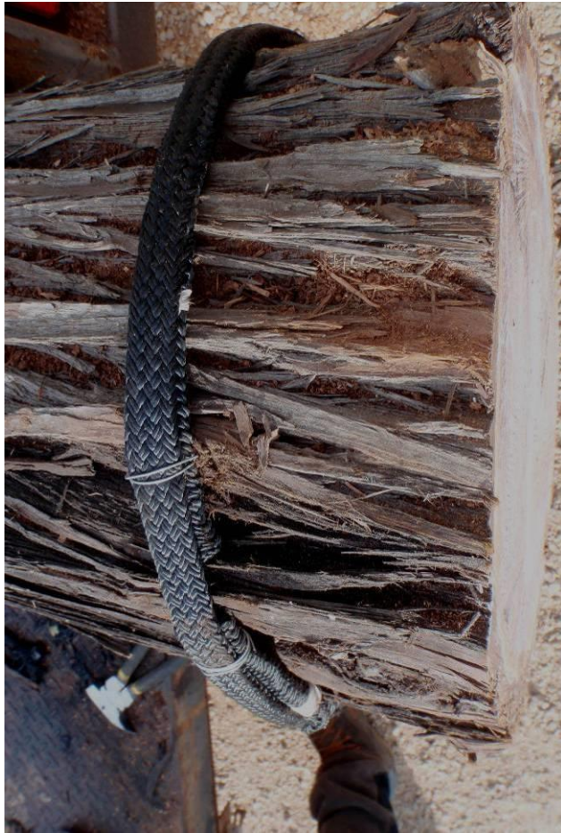
Figure 35. Strapping at end of Callitris log to further reduce splitting.
