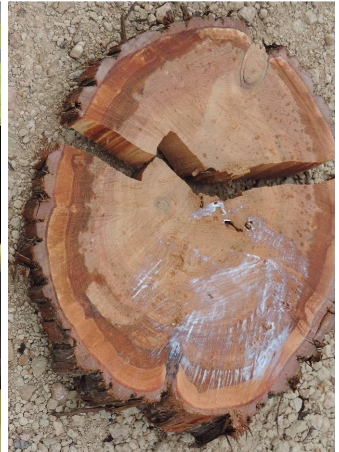
Figure 34. Split end grain biscuit from Callitris log five minutes after cutting.
