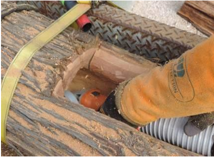
Figure 5. Large Arbortech® blade attached to AEG Angle grinder used to sculpt internal surfaces of nest-box. Note gray dust cover extending beyond the work area to protect the angle-grinder motor.
