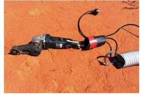
Figure 7. Arbortech® mini grinder with improvised dust cover (light grey) and handle removed. The red tape holds a rubber strip fitted to ensure an airtight fit.
