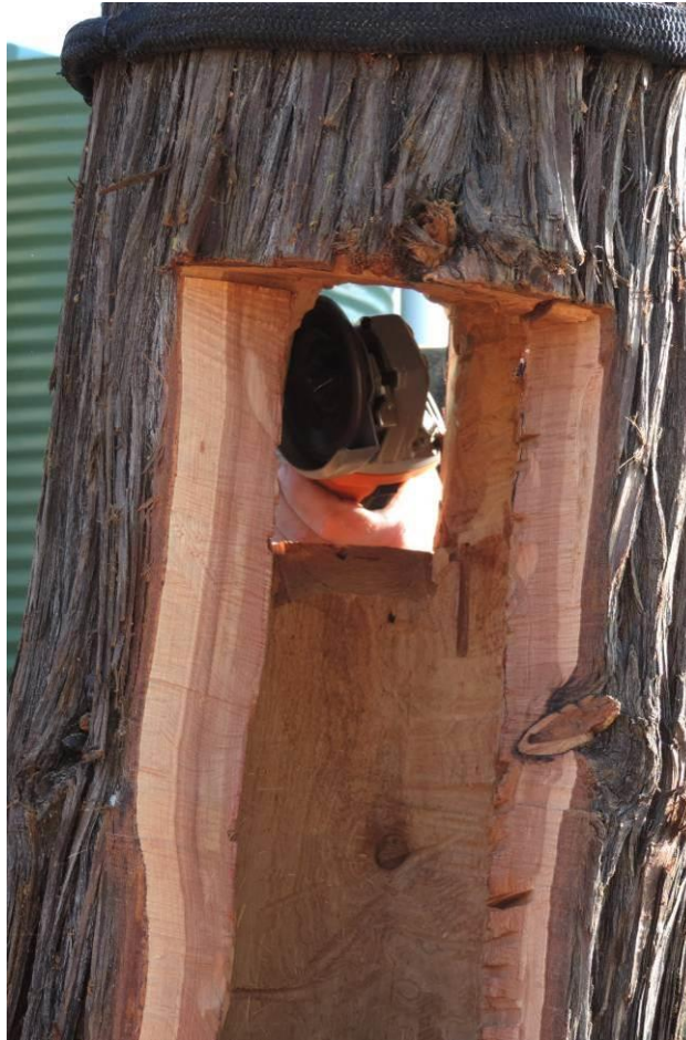
Figure 51. Arbotech being used to smooth-off and form external entrance features.
