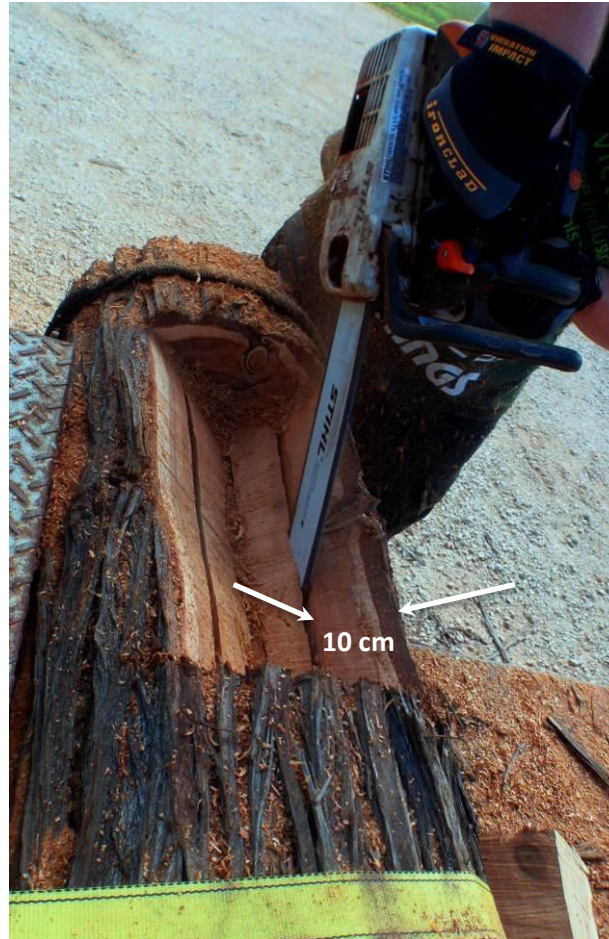
Figure 39. To hollow-out the cavity, first make outer cuts to allow the cavity walls to be at least 10 cm thick. Then further slits can then be cut to the appropriate depth.
